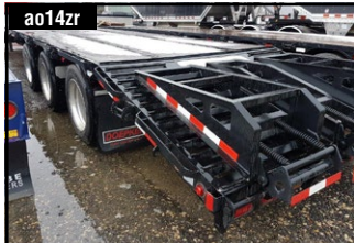
ao14zr 2016 DOEPKER 53' Drop Deck, Fixed Beavertail & Flip Ramps, CS Toolbox, 255/70R22.5. Stk # G1035276
